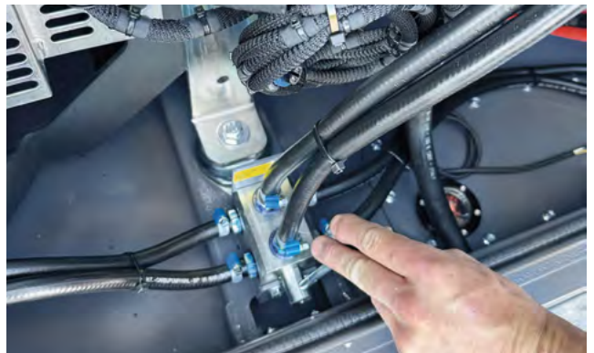
3-way valve for external tank connection
