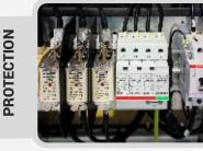
Up to 250kVA ±15%: An automatic circuit breaker is mounted on the regulation circuit to protect against overload and short circuit on the voltage regulator. The auxiliary circuit is protected by **fuses**. Overvoltage protection: Class II output **surge arrestor**.
