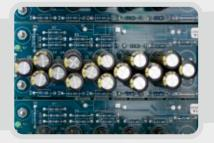
Output voltage reset to the minimum value in case of blackout by means of **supercapacitors** banks in order to ensure the correct shutdown.
