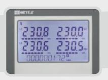
The digital measuring instrumentation consist of two (input & output) **multi-task digital line analyser**.
