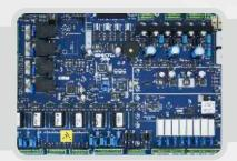
The control logic, performed on the **true RMS value**, is based on two **2-way DSP microprocessor** and supervised by a third **bodyguard microprocessor** with Ortea dedicated firmware.
