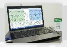
Monitoring activities can be run remotely by installing on a a PC (connected to the stabiliser via Ethernet) the **STABIMON software** provided with the unit. It is also possible to communicate with the stabiliser with the **Modbus TCP/IP** protocol.
