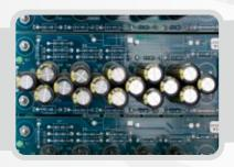
Output voltage reset to the minimum value in case of blackout by means of **supercapacitors** banks in order to ensure the correct shutdown.
