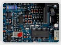
Control logic based on digital **microprocessor** with Ortea dedicated firmware. All the Vega, Antares and Orion stabilisers are fitted with the **same control card**, thus simplifying maintenance operations and spare parts storage.
